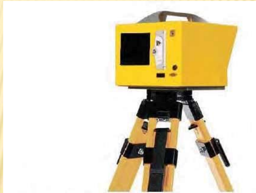
TLS ILRIS 3D (Picture extracted from: www.Optech.ca )
