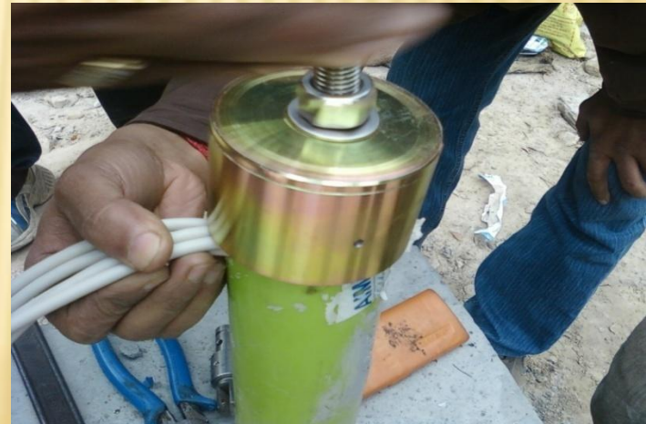
Top Cap Assy. with wires through Groove
