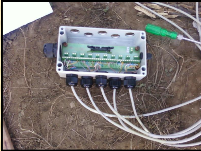
IPI Sensors connected to JCB
